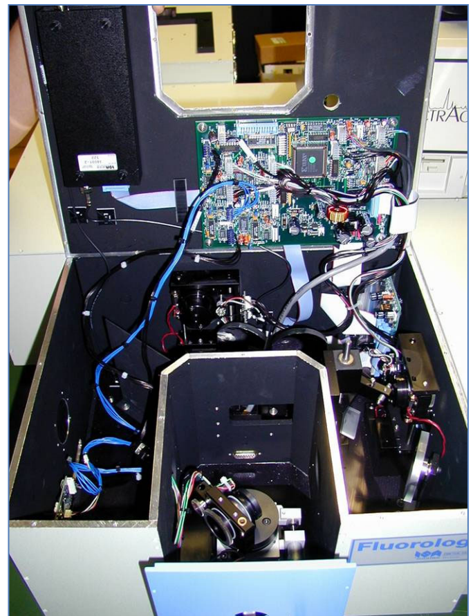
Figure 3: Installation of the "Rotating" sample holder in the Fluorolog3
