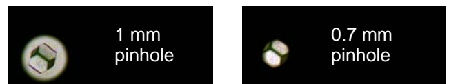
Fig. 7. A glucose isomerase crystal (70 \mu\text{m} across) using different pinholes in the emission path, and a 10 \times objective.
