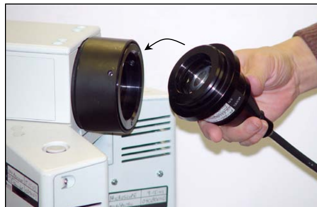
Fig. 3. Attaching the excitation fiber-optic bundle to the microscope's white-light source.
