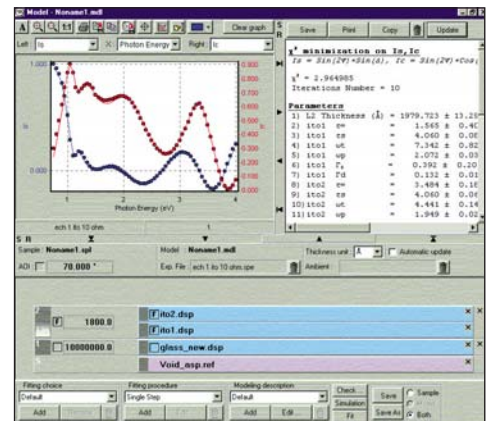
ITO graded layer model taking into account backside reflections
